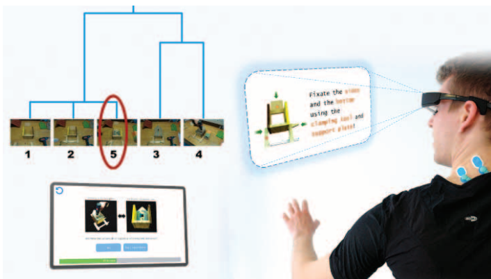
Fig. 1 Special software from cognitive sciences (lower left) enables the prediction of human action errors (upper left) for individualised user assistance, e.g. using intelligent smart glasses (right)
